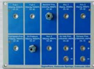
The modular sensor box allows for additional 10-channel pressure panels (shown) and additional 16-channel temperature panels. Extra transducers are sold separately.
