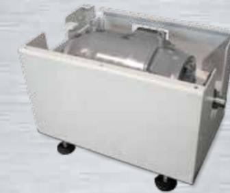
The AC Motoring Cube brings emissions level test data the CycleDyn. It allows you to perform R&D economically prior to final certification. The AC cube will simulate inertia, rolling losses and aerodynamic effects with the help of an advanced motor controller and WinDyn. Perform coast downs and evaluate parasitic losses or use SuperFlow's drivers trace software to perform emissions drive cycles.
