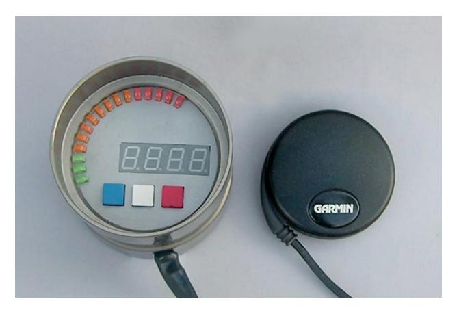
There are only two (2) wires to hook up. Red wire to 12V Dc Switched Power and Black Wire to Ground. There is nothing to calibrate or set.
