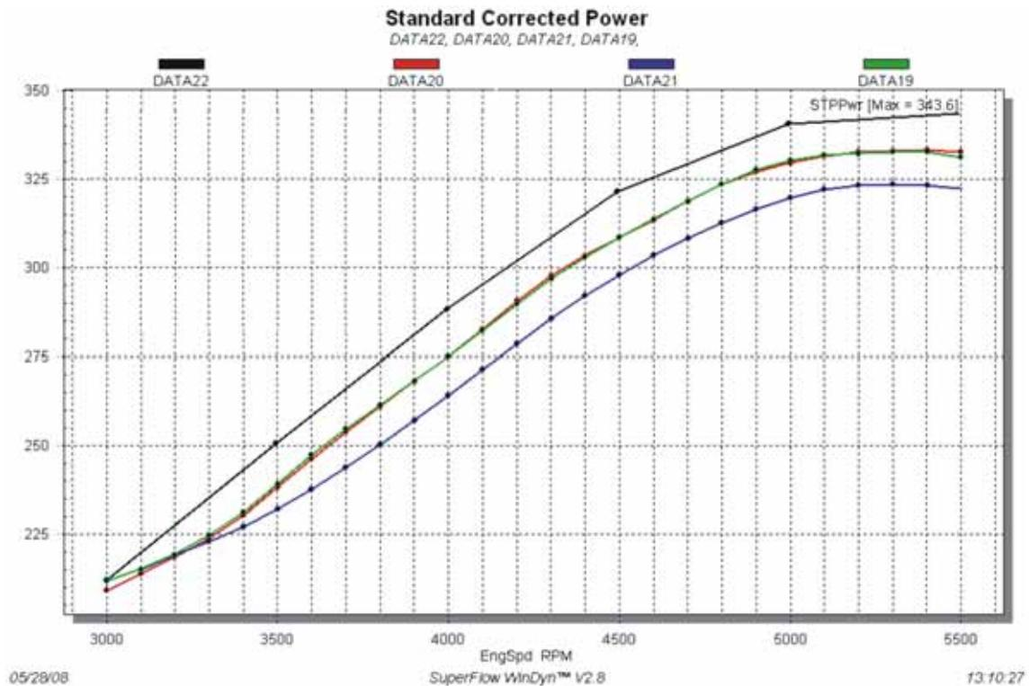
In the graph above, the black line is a 500-rpm step test. It makes the most power, from 3,000 to 5,500 rpm.
