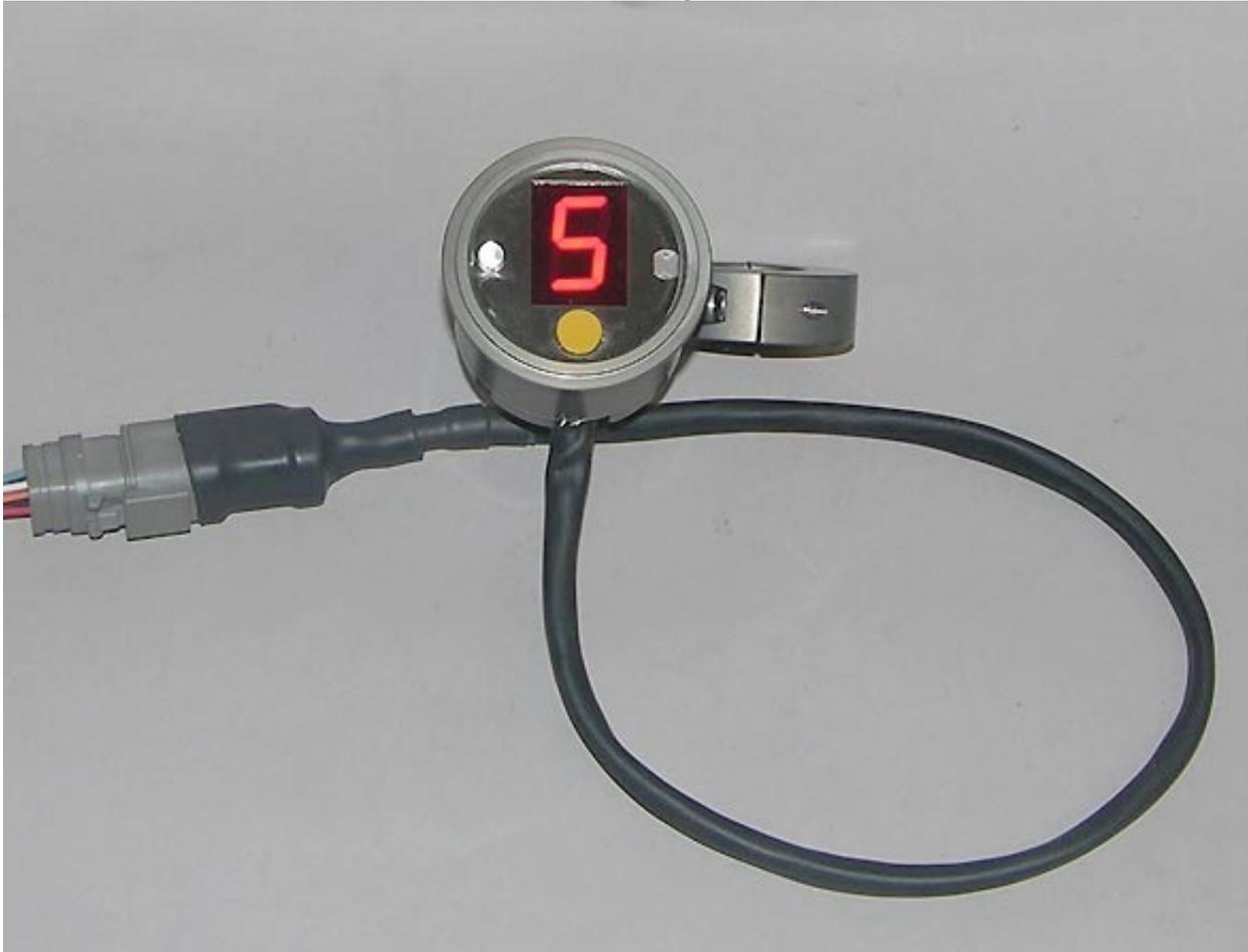
The gauge is cnc machined billet enclosure with a back mounted 5/16” x 18 buttonhead cap screw. A total of four to seven wires are used to hook up the RSR Bonneville Gear Indicator.
