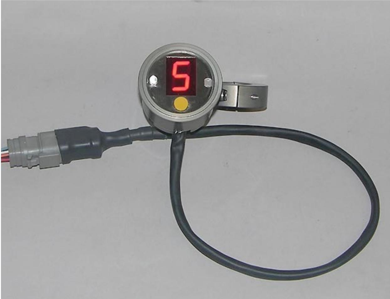
First step is to mount the gauge where you can easily see it in normal vehicle operation. A gear position indicator is meant to be used, not just because it is a neat accessory that looks cool. Part # 06-1028. 1.0" or 1.25" cnc machined handlebar clamps are standard.
