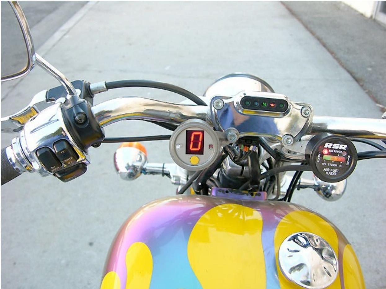
During daylight operation the display needs to be at full brightness. At night the display needs to be dimmed to avoid a blinding distraction.
