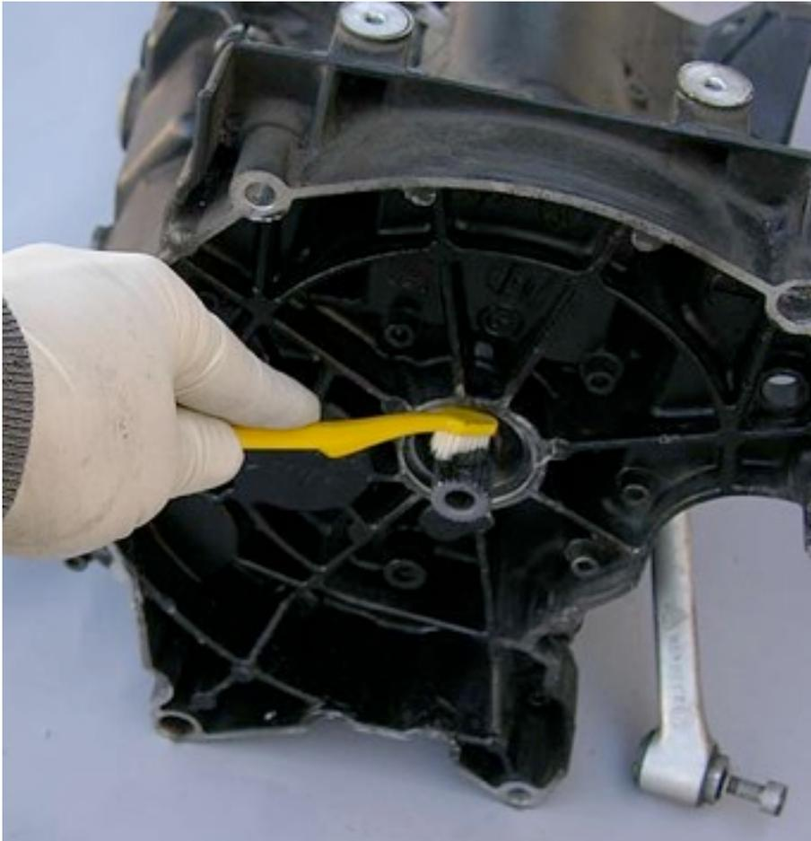
Rotate the shaft to insure all the surface is coated. When you are finished it is a good idea to either clean the toothbrush or place it in the provided ziplock bag as the grease will stick to everything.
