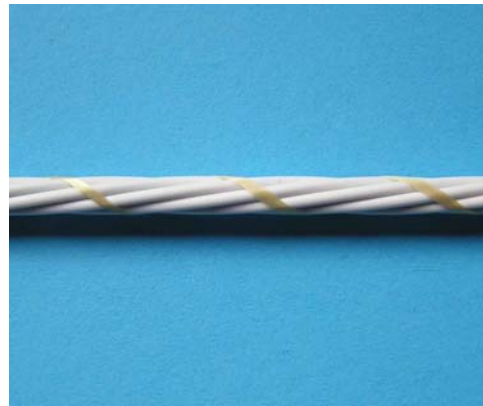
NOT ACCEPTABLE Lay length of Binder too long
