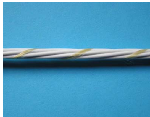
NOT ACCEPTABLE Binder wrapped in wrong direction
