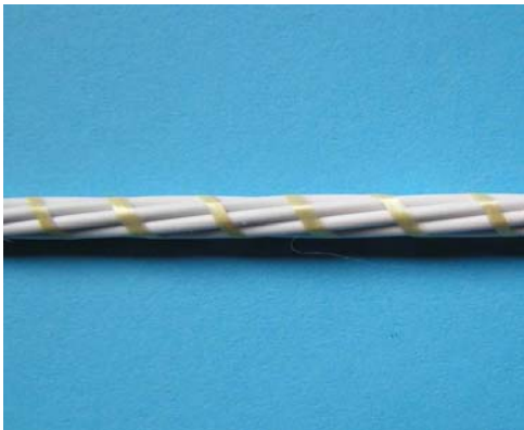
NOT ACCEPTABLE Lay length of Binder too short
