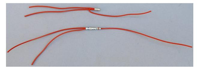
Top splice is a Parallel Stub Splice
