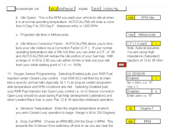
Drop In RPM. Typically this is 250 RPM less than the Drop In RPM.
