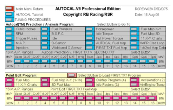
AUTOCAL.V6 gives you the ability to Predict, Analyze, and Edit your RSR Fuel Injection's Programs. AUTOCAL.V6 will generate Autocal.TXT files (complete ECU Calibrations) and transfer them to the FUEL Directory with the simple selection of one button. The AUTOFMP File Utility which resides between the FUEL and AUTOCAL.V6 programs will translate these .TXT Files into .FMP files that can be read by the FUEL Program, and FMP Files into .TXT files for analysis or editing in AUTOCAL.V6.
