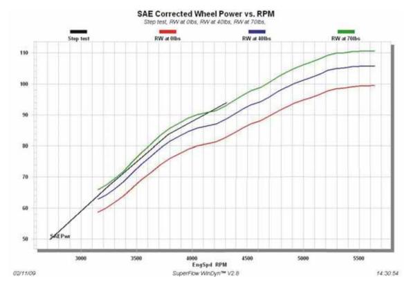
In the example above, we show the effects of "estimating" vehicle inertia. These tests were performed on a V-Twin motorcycle with a large 280-mm rear wheel mounted. The red, blue, and green lines represent a rapid inertial type sweep test approximately 3.5 seconds in duration. The
