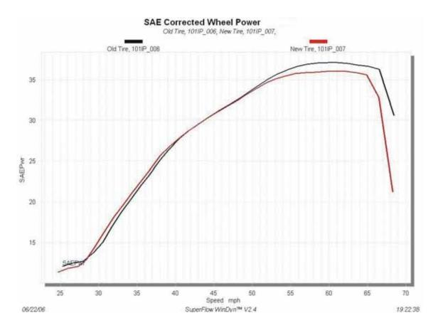
The inertia power calculation is based on two measurements taken by the dynamometer: roll speed in mph and acceleration in mph per second, or G's. In this case, the new tire had a smaller diameter by about .5 inches. This should have caused the acceleration rate to be quicker for any given engine speed (rpm).
