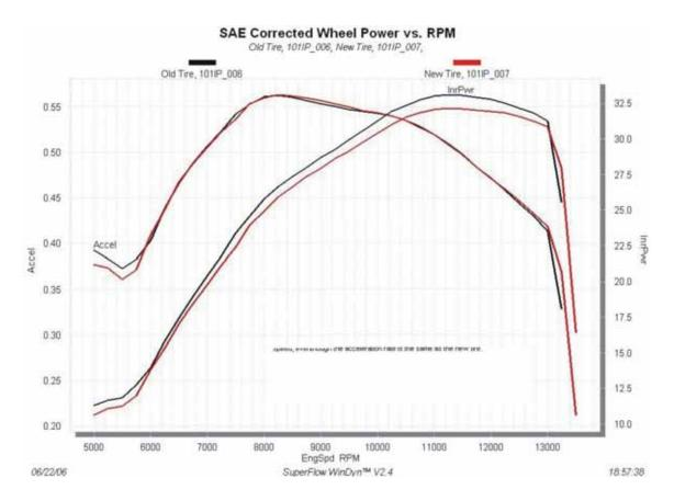
This graph clearly depicts the change in gearing that occurred from the smaller diameter new wheel/tire combo.
