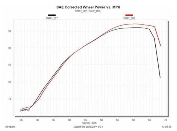
This is a very good comparison chart demonstrating how a change to a different wheel and tire on a motorcycle can affect the power measured. In this case, test 6 was an inertia run with a 25.6" Kenda tire that was pretty worn out.
