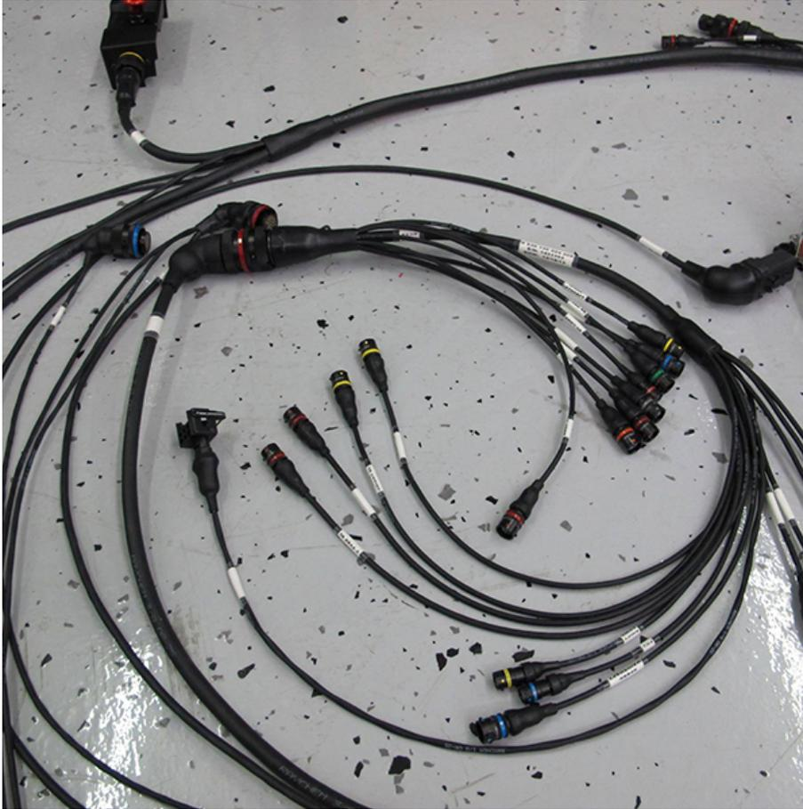
Gibson says that even for a grassroots race application, he would stick with the better Tefzel wire, but there are cases where TXL may be used. “I would definitely use the Tefzel either the 55-8 from Raychem or a Mil-spec equivalent. The only reason I would ever use the TXL/GXL is to have connectors that need to be sealed in the back. The Tefzel is so thin that it may not seal the back of the OEM connector, but generally, you want to try to put boots on stuff.”
