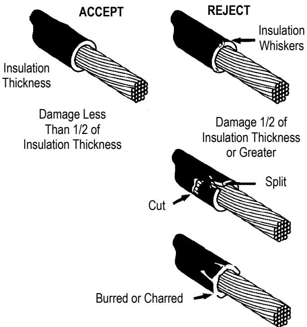
Check to see if the stripping tool or machine has cut or nicked any of the wires. If you see nicked wire you must cut and re-strip the wire before crimping to be sure that the amount of current that can be carried is not reduced.
