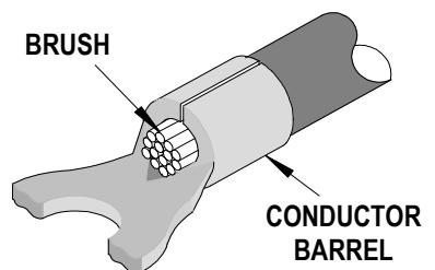
contact side of the terminal. This helps ensure that mechanical compression occurs over the full length of the conductor crimp. The conductor brush should not extend into the contact area.
