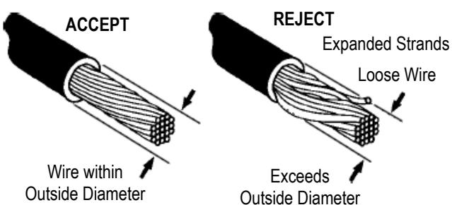
Check the insulation to ensure that there has been a nice clean cut. Wires with damaged insulation should not be used.
