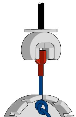
If results of a pull force tests are within an allowed range, it assures that proper crimp force has been applied during crimping. It is crucial as, when making a crimp, enough force must be applied to break down the layer of non-conductive oxides that may build up on the stripped conductor and the tin-plating on the inside of the terminal grip. This is necessary to provide a good metal-to-metal contact.
