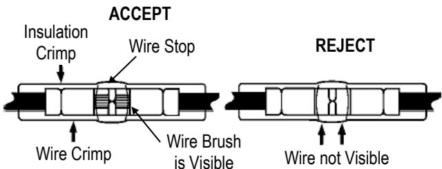
1. Be sure that the wire is visible in the inspection window so that there is evidence of a good crimp. See Butt Connector above.
