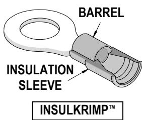
4. The Avikrimp™ has a color-coded sleeve, which provides insulation as well as an insulation grip. The insulation is made of Nylon, and has a secondary tin-plated brass sleeve added. This brass support sleeve is crimped around the wire
