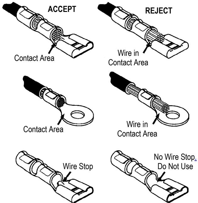
1. Be sure that no wire strands extend into the contact area of the lug or terminal.
