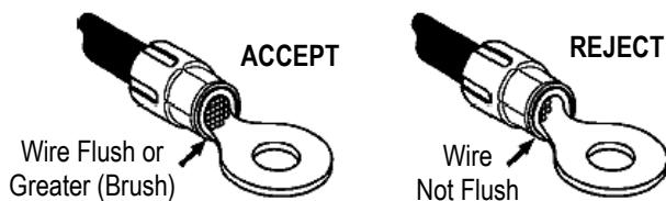
1. Be sure that the wires are either flush with the end of the conductor barrel or extend past the barrel.
