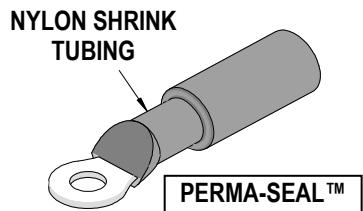
8. The Eyelet can be used in place of standard compression terminals because it is deep drawn from CDA-110 electrolytic pitch copper and then tin-plated for corrosion resistance. It has a seamless barrel with a flared barrel entry. It is available in wire range 8 to 500 MCM.
