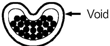
If the die presses too tightly the individual strands can be squeezed and elongated. This can cause a weak point in the conductor, cause the wire to break at a lower than allowable tensile strength, and/or create a heat rise across the joint because of lower cross-section and increased resistance.
