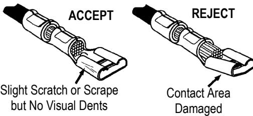
1. Be sure that the contact area is not dented or crushed.
